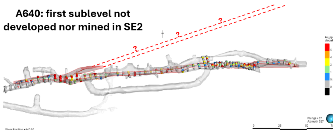
Figure 3. Horizontal plan-view sections of orebody A at three elevations, illustrating the current drilling status and interpreted continuity of the A/SE2 lens: (a) A640 level — first sublevel of the A/SE2 body that remains undeveloped and unmined; (b) A420 level — last sublevel of the ASE2 body that remains undeveloped and unmined; (c) A400 level — first sublevel where the SE2 body was developed and mined. Each section displays the interpreted geological wireframe of orebody A, existing drillhole assays with positive gold results, and the interpreted continuity of the SE2 lens.
